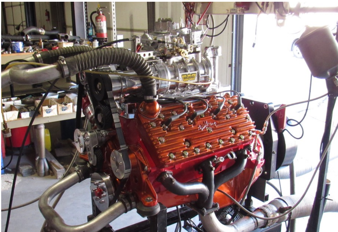
Figure 2. Bonner 293 Cu.In. Flathead with Roadrunner Supercharger
