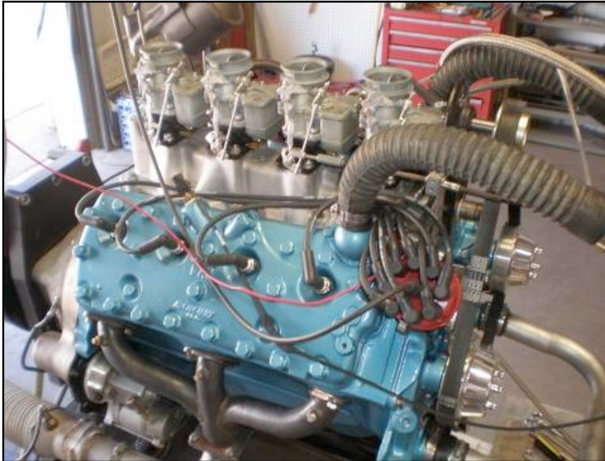
Four Stromberg 97's on a Weiland Manifold
