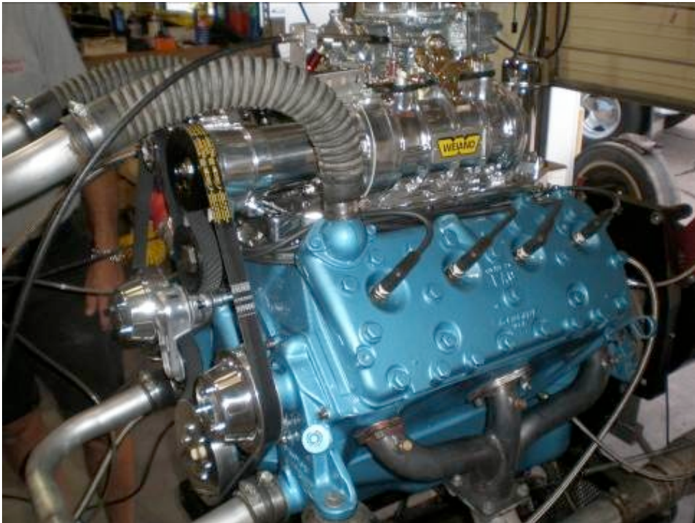
Roadrunner Kit with a Weiland 142 Blower and a Holley Street Avenger 4-bbl installed
